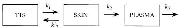
Fig. 1. Schematic representation of the three-compartment model and the respective rate constants implied in mass transfer between the different compartments, indicated by k_1 , k'_1 , k_2 and k_3 .
